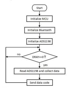
Fig. 3. Flow chart of data acquisition and wireless transmission module
