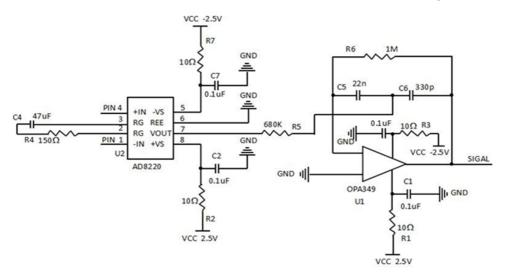
Fig. 1. Circuit diagram of enlargement and filtering
