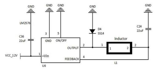
Fig. 2. LCD power supply
